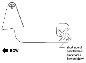
Figure 2-13: Orienting the Paddlewheel
